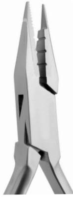
66-5100 Jarabak Pliers Excellent for precise wire bending and forming of loops. The fine serrations on the square beak and three precision grooves permit accurate and intricate bends and
