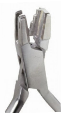
66-5103 Loop Tie Back Plier Four-step plier automatically forms loops on wire up to .020" with one motion. Closing loops are easily made to desired height.
